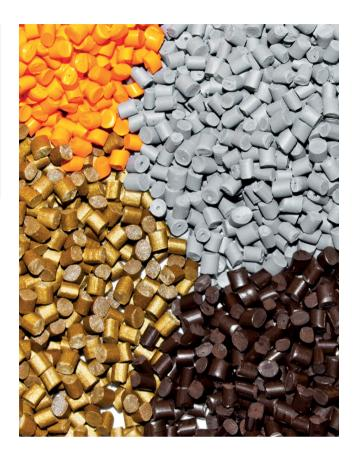
For optimal precision, it is essential to stabilise the temperature of the polymer prior to measurement; usually at 40°C, which is the same temperature as the magnet.
